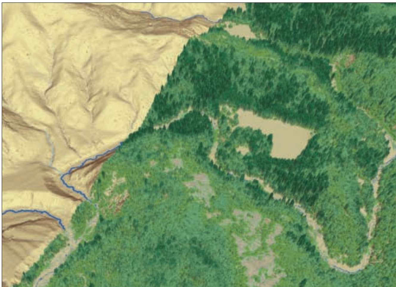
Figure 3. Digital elevation maps (DEM) showing a section of the Angelo Coast Range Reserve, Mendocino County, CA. This 3D visualization was constructed from airborne laser swath mapping data, processed into canopy DEM, bare-earth DEM, and a stream channel network. The canopy is colored by extracting vegetation height from the difference between canopy and bare-earth DEMs. The stream channel network was draped onto the bare-earth and colored by drainage basin size. This type of dataset can provide a detailed template for launching an iterative cycle of investigation that integrates mapping, monitoring (Figure 2a), tracing, experimentation (Figure 2b), and modeling and visualization (Figure 2c). Data flown and processed by the National Center for Airborne Laser Mapping (NCALM), funded by the National Center for Earth Surface Dynamics (NCED).
