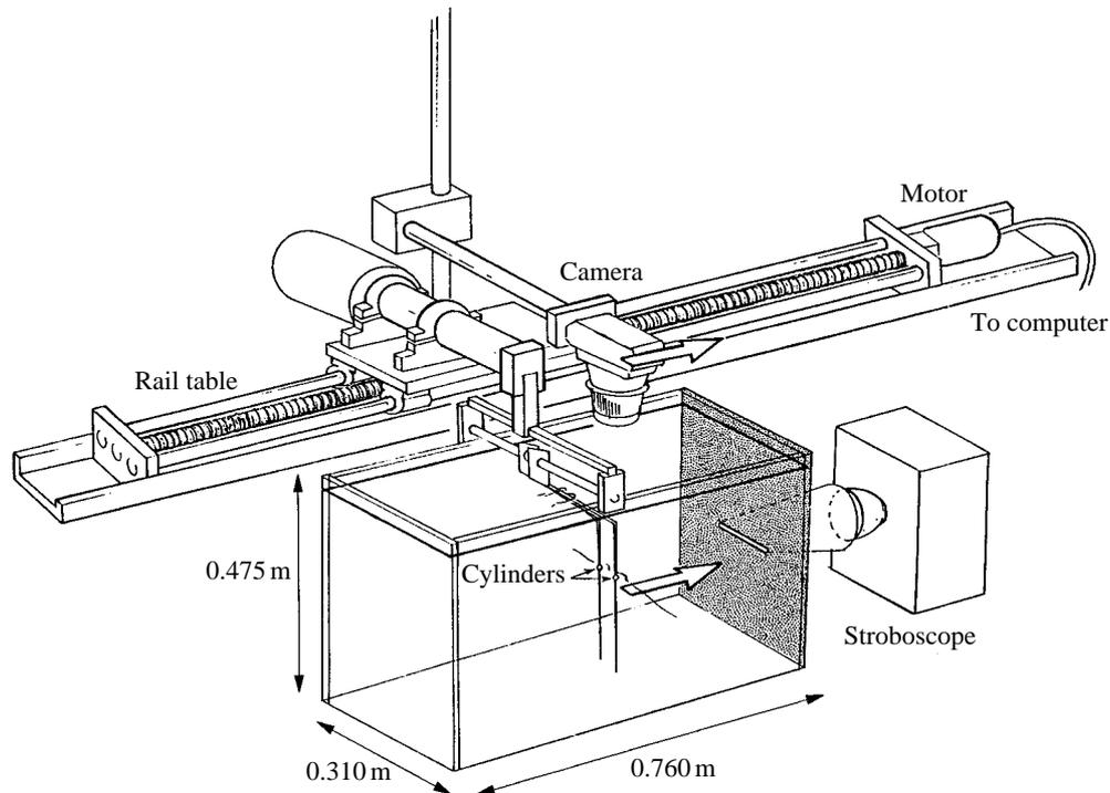
Fig. 2. Experimental apparatus for recording the movement of flow markers past the cylinders. The camera was stationed above, and moved with, the cylinders (movement indicated by arrows). This movement was driven by a motorized rail table controlled by a computer. Flashing light from a stroboscope entered the tank through a horizontal slit.
