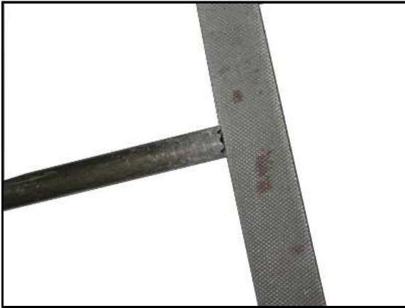
Fig. 2 shows the notches being cut in the end of the vacuum tube.
