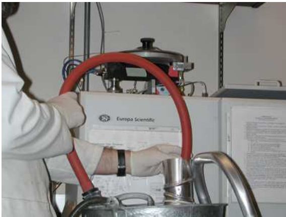
Fig. 4 shows the metal pale and suction device in place in front of the elemental analyzer.
