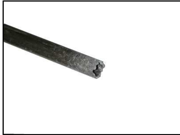
Fig. 3 shows the finished notches at the end of the vacuum tube.
